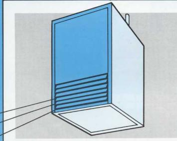
The Uni-Pak unit heater's interchangeable louvers and panels permit air to be discharged horizontally or downward to meet area heating requirements. Panels can be field changed easily as needed.
